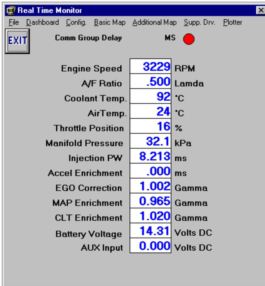
The real Time Monitor allows the user to view the operation of the controller while the controller is operating. This allows the user to gauge the level of tuning required, and to troubleshoot the system after installation, or if a problem arises later.
