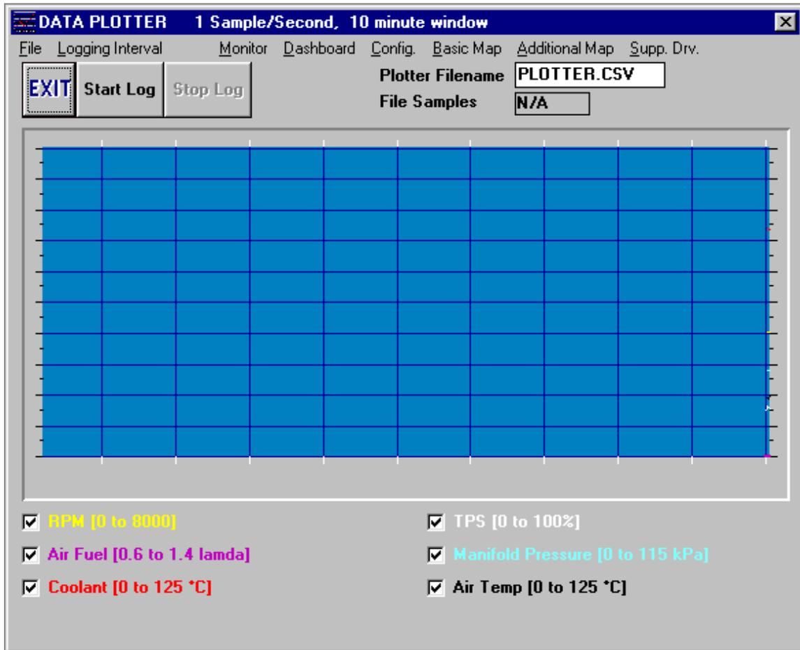
The Data Plotter is a tool to monitor performance trends and to plot or log sensor data into a spreadsheet file for later evaluation.
