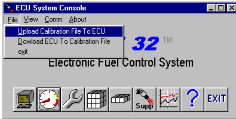
If the user is happy with a given configuration stored within the engine controller, or if the user wishes to save a reference "snapshot" of the data in the engine controller, the entire controller data-set can be stored off to a calibration file on the PC. The file may then be read, and restored into the engine controller at a later time. This can be useful to maintain a set of configurations that go with different engine modifications, or even different engines.
