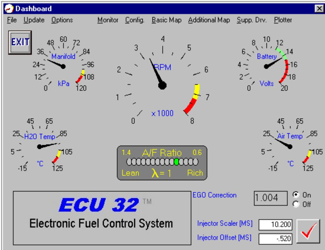
This is another monitor only feature that allows a graphical representation of the engine tachometer, air and coolant temperature sensors, battery voltage and manifold pressure. Also provided is a simulated LED Lambda meter for monitoring the air fuel mixture.
